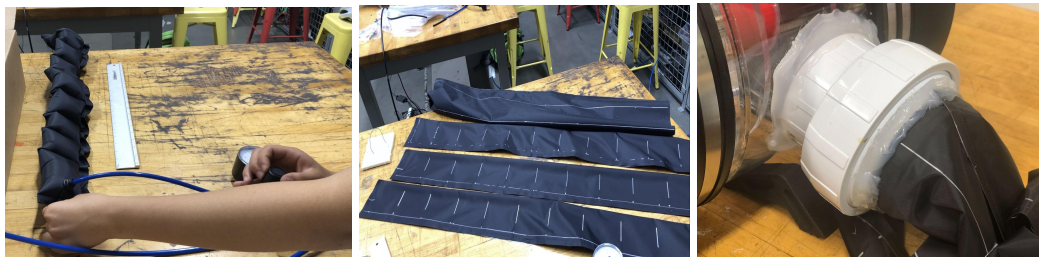
Figure 8.2.102 - Vine Body Construction (reprinted with permission from vinrobots.org)
